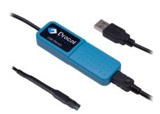
The TRH200 is designed for environmental temperature and humidity acquisition. Its exposed sensor allows for more precise temperature measurements of hard surfaces. Thanks to its factory-calibrated, linearized, and temperature-compensated digital sensor chip, the TRH200 is field interchangeable. With its precision electronics, minimal variations in temperature and humidity can be detected.
